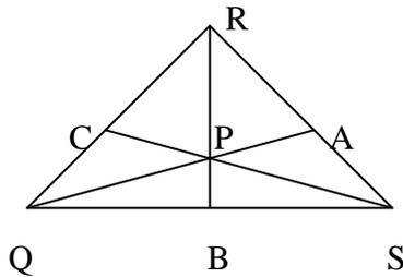
4. In  $\triangle QRS$  with medians  $\overline{QA}$ ,  $\overline{RB}$ , and  $\overline{SC}$  are concurrent at point P. If  $RP = 6$ . Find PB.
